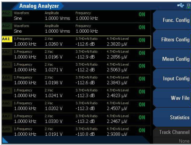
Figure 1. The U8903B's GUI, showing 8 analyzer channel measurements.
